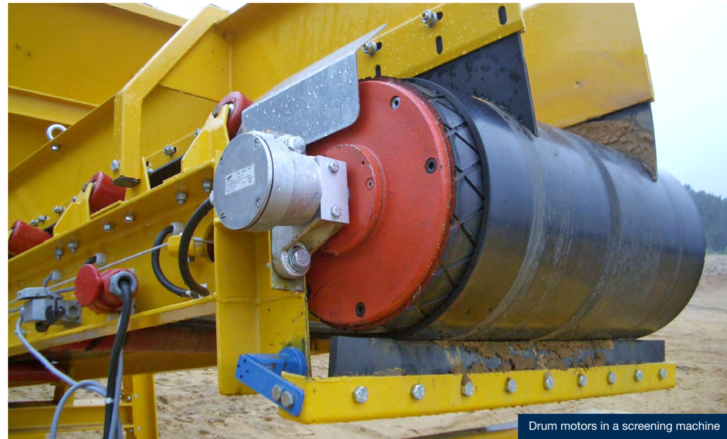
Drum motors in a screening machine
